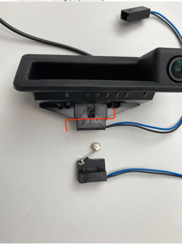
2. Insert the handle camera combination in the original handle slot. Previously removed piece will allow to fit it.
