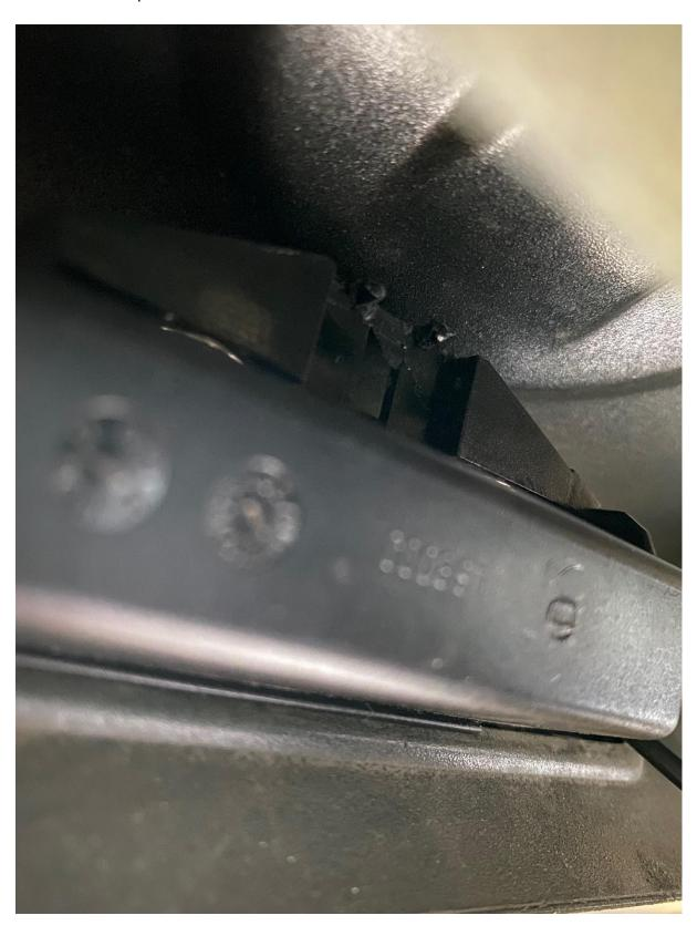
3. Put some glue on the removed actuator and fix it back to its position on the guiding rivets. Test the actuator.
